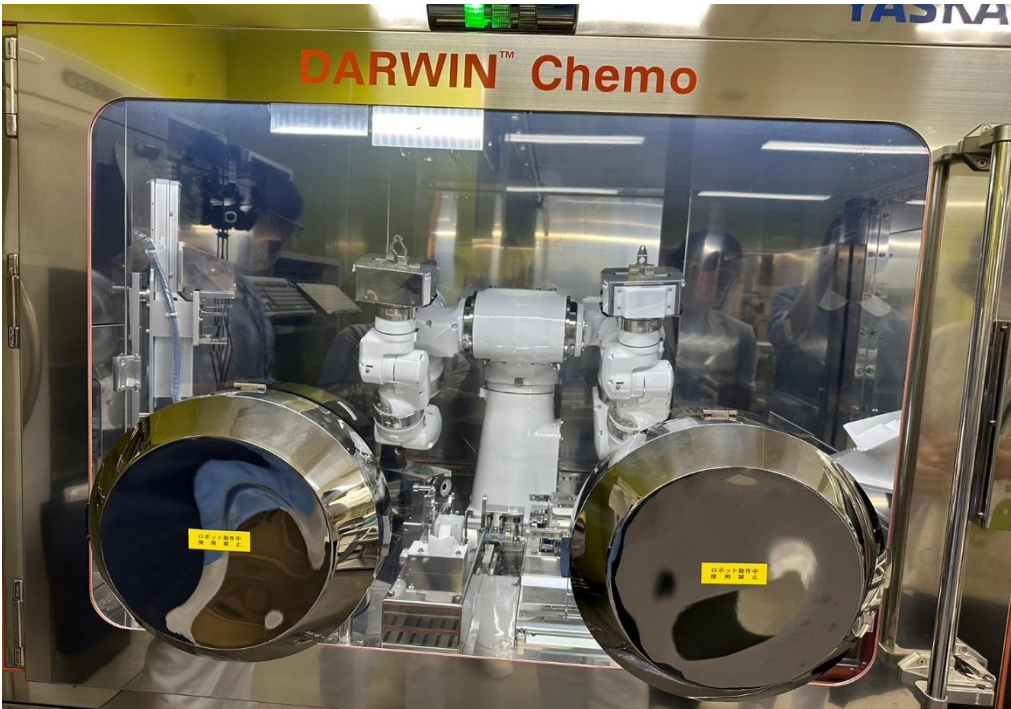
This is a machine used for compounding cancer medication. The pharmacist informed us that there are only three machines like this, and one of them is located here at OMPU hospital.
